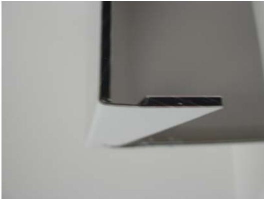
Distorted Flat rout folded 90°
