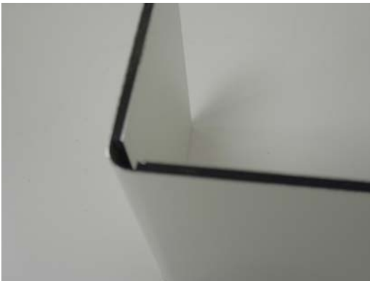
Alucobond® Corner with Flat Rout
