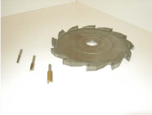
Flat Router Bit and Saw Blade
