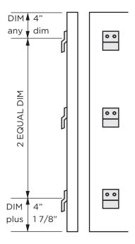
For a typical 8' high x 4' wide panel, customers mount the continuous lengths along the wall at 3 different heights parallel with the floor. These are secured to studs at 16" on center or to blocking at 8" on center. The shorter panel clips are secured to the back of the panel every 12-15" horizontally.
